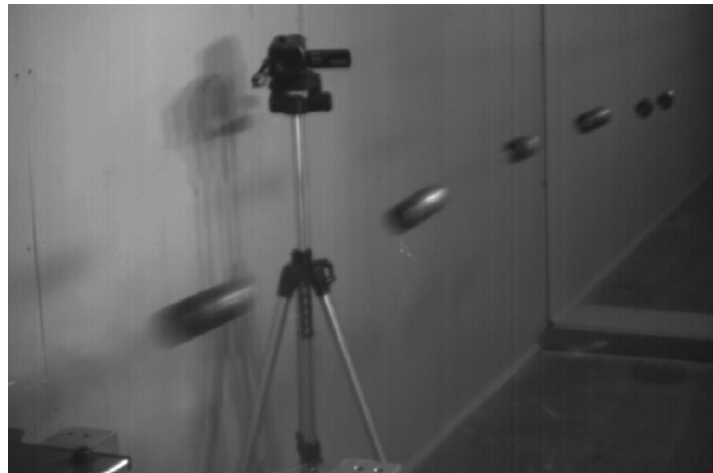
40mm rounds fired at over 10,000rpm
